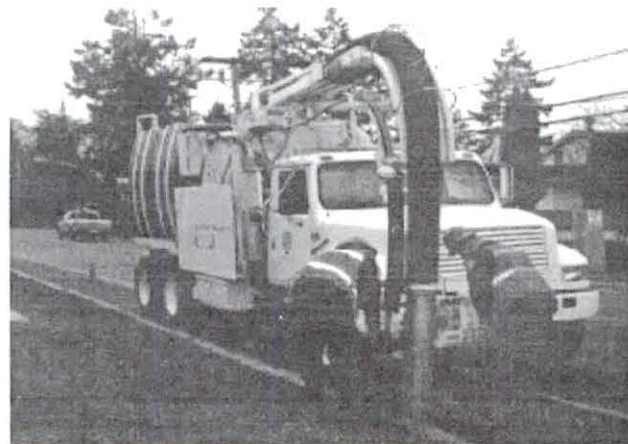
A Vactor truck is used to clean out catch basins and storm lines to improve surface water drainage.
